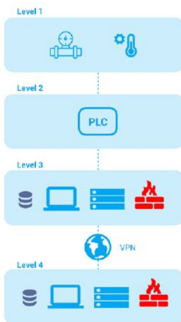
Power Plant Network Architecture
